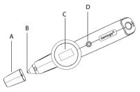
A - Cap B - Detection Tip C - Display Area D - On/off button
